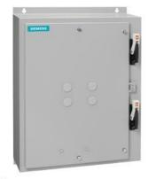
Duplex starter w/o alternator, Size 1, Three phase full voltage, Solid-state overload relay, OLR amp range 5.5-22A, 240V 50Hz / 277V 60Hz coil, Combination type, Two 25A circuit breakers, Encl NEMA type 4X 304 S-Steel, Water/dust tight noncorrosive
