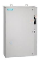
Non-reversing motor starter, Size 3, Three phase full voltage, Solid-state overload relay, OLR amp range 25-100A, 240V 50Hz / 277V 60Hz coil, Combination type, 125A circuit breaker, Encl NEMA type 4X 316 S-Steel, Water/dust tight noncorrosive, Extra-wide enclosure
