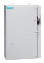
Non-reversing motor starter, Size 2 1/2, Three phase full voltage, Solid-state overload relay, OLR amp range 25-100A, 24VDC coil, Combination type, 100A fusible disconnect, 100A/250V fuse clip, Enclosure NEMA type 4/12, Water/dust tight for outdoors, Standard width enclosure
