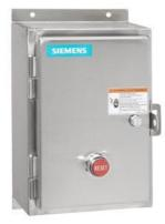
Non-reversing motor starter, Size 3 1/2, Three phase full voltage, Amb. compensate bimetal OLR, Contactor amp rating 115A, 24VDC coil, Non-combination type, Encl. type 4X 304 S. Steel, Water/dust tight noncorrosive
