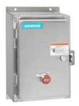
Non-reversing motor starter, Size 2 1/2, Single Phase, 2-Pole, Amb. compensate bimetal OLR, Contactor amp rating 60A, Non-combination type, Encl. type 4X 304 S. Steel, Water/dust tight noncorrosive
