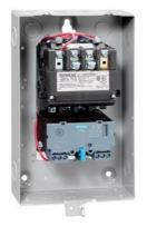
Non-reversing motor starter, Size 1, Single phase full voltage, Solid-state overload relay, OLR amp range 0.75-3.4A, Non-combination type, Enclosure type 1, Indoor general purpose use, Standard width enclosure
