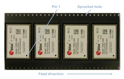
Figure 5: Orientation for TOBY-L2 modules on tape
