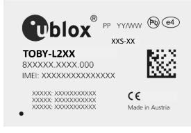
Figure 7: Example of TOBY-L2 series module label
