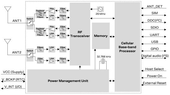
Figure 1: TOBY-L2 series block diagram
