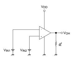
$$V_{IN1} = \frac{V_{DD}}{2} - 0.05V$$
