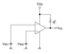
$$V_{IN1} = \frac{V_{DD}}{2} + 0.05V$$
