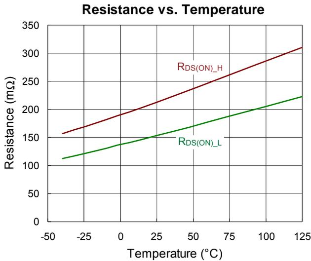
Figure 14. RTQ2131B R<sub>DS(ON)</sub> vs. Temperature
