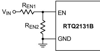
Figure 13. Resistive Divider for Under-Voltage Lockout Threshold Setting
