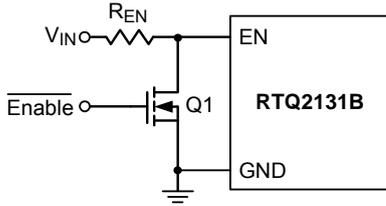
Figure 12. Logic Control for the EN Pin
