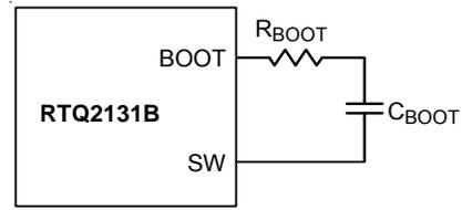
Figure 9. External Bootstrap Resistor at the BOOT Pin
