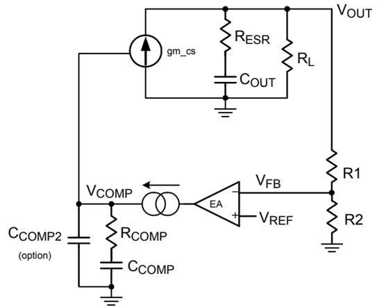
Figure 7. Simplified Equivalent Circuit of Buck with PCMC
