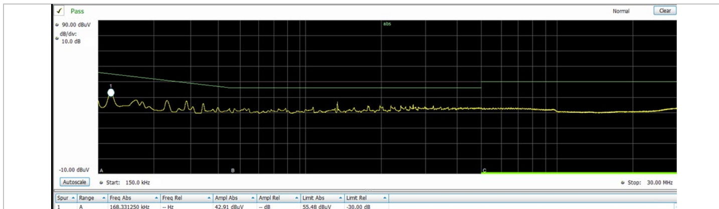
EMI; Conducted CISPR 22; Peak vs. Average Limit; L2/Neutral; 100Vac 24Vdc @ 25A
