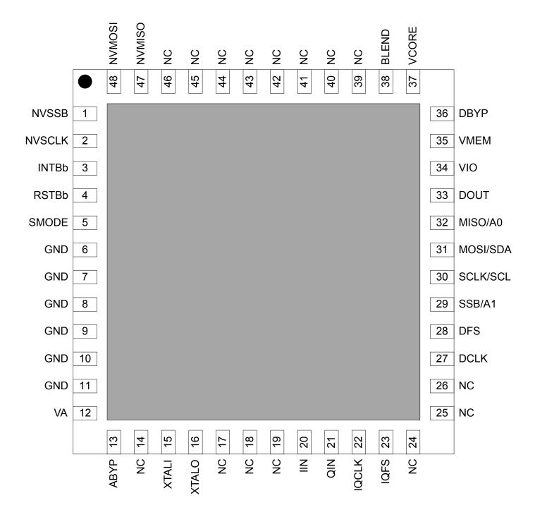
Figure 1.1. Si4693 Pinout Diagram
