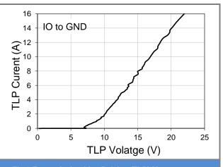
Fig.2 Transmission Line Pulsing (TLP) Measurement
