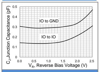
Fig.1 Typical Junction Capacitance
