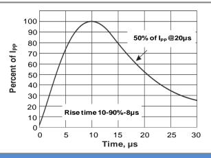
Fig.4 8/20μs Pulse Waveform
