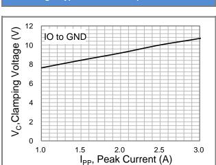
Fig.3 Typical Peak Clamping Voltage(8/20μs)
