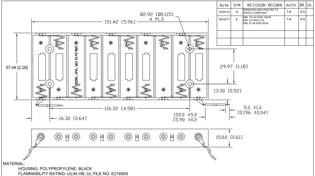
TEMPERATURE RANGE: -10°C to +100°C SPRINGS: SPRING STEEL, NICKEL PLATED
