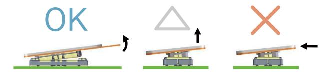
3. If the FPC does not have sufficient rigidity, solder stripping or connector breakage may occur.
