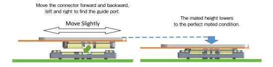
3.In the engaged state, the connectors are parallel to each other, and the connectors cannot move forward, backward, left, or right. Complete mating from this state.
