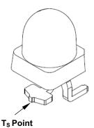
$T_S$  can be easily measured by mounting a thermocouple on the soldering joint as shown in Figure 15, while  $R_{\theta J\text{-}S}$  is provided in the data sheet. Verify the  $T_S$  of the LED in the final product to ensure that the LEDs are operating within all maximum ratings stated in the data sheet.
