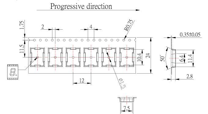
Note: Tolerances unless mentioned ±0.25mm. Unit = mm **Packing Process**
