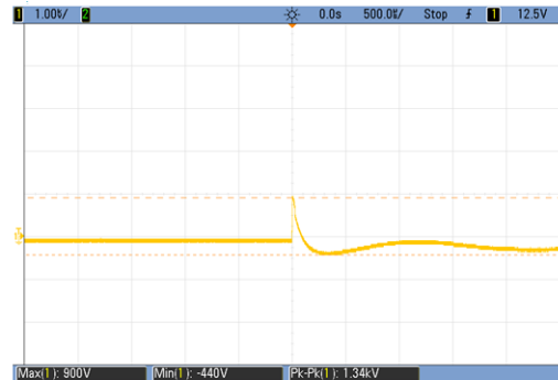
Output voltage waveform (0.9 KV)
