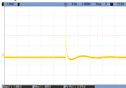
Input voltage waveform (Differential mode 1.99KV)
