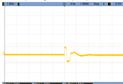
Output voltage waveform(0.71 KV)
