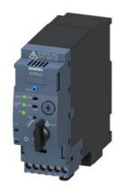
SIRIUS Compact load feeder DOL starter for IO-Link 690 V 24 V DC 8...32 A IP20 Connection main circuit: plug-in, without terminals Connection control circuit: screw terminal
