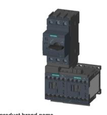
FUSELESS LOAD FEEDER REVERSING OPERATION, 400 V AC, S00 0.28 TO 0.40 A 3K W, 110/120 V AC 50/60 HZ SCREW TERMINAL FOR STANDARD RAIL MOUNTING, TYPE OF COORDINATION 2, IQ = 150 KA (ALSO FULFILLS TYPE OF COORDINATION 1) 1NC (CONTACTOR)
