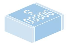
Smaller size components will be marked with a 2-digit code in accordance with EIA-198 marking requirements.
