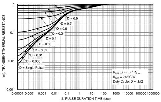
Figure 13. Transient Thermal Resistance
