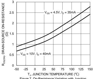
Figure 7. On-Resistance Variation with Junction Temperature
