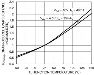
Figure 6. On-Resistance Variation with Junction Temperature
