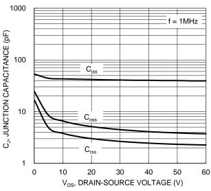
Figure 10. Typical Junction Capacitance
