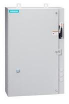
Non-reversing motor starter, Size 0, Three phase full voltage, Solid-state overload relay, OLR amp range 3-12A, Combination type, 10A circuit breaker, Encl NEMA type 4X 304 S-Steel, Water/dust tight noncorrosive, Extra-wide enclosure
