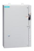
Non-reversing motor starter, Size 3, Three phase full voltage, Solid-state overload relay, OLR amp range 25-100A, 24VAC 50-60Hz coil, Combination type, 100A fusible disconnect, 100A/250V fuse clip, Encl NEMA type 4X 304 S-Steel, Water/dust tight noncorrosive, Standard width enclosure
