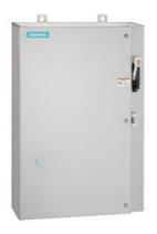
Non-reversing motor starter, Size 2 1/2, Three phase full voltage, Solidstate overload relay, OLR amp range 25-100A, 240V 50Hz / 277V 60Hz coil, Combination type, 100A fusible disconnect, 100A/250V fuse clip, Encl NEMA type 4X 304 S-Steel, Water/dust tight noncorrosive, Extra-wide enclosure
