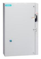
Non-reversing motor starter, Size 2 1/2, Three phase full voltage, Solid-state overload relay, OLR amp range 25-100A, Combination type, 100A fusible disconnect, 100A/250V fuse clip, Enclosure NEMA type 1, Indoor general purpose use, Extra-wide enclosure
