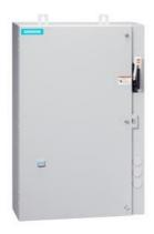
Non-reversing motor starter, Size 1, Three phase full voltage, Solid-state overload relay, OLR amp range 3-12A, 24VAC 50-60Hz coil, Combination type, 30A fusible disconnect, 30A/250V fuse clip, Enclosure NEMA type 4/12, Water/dust tight for outdoors, Extra-wide enclosure
