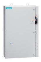
Non-reversing motor starter, Size 0, Three phase full voltage, Solid-state overload relay, OLR amp range 3-12A, Combination type, 30A fusible disconnect, 30A/600V fuse clip, Enclosure NEMA type 4/12, Water/dust tight for outdoors, Extra-wide enclosure
