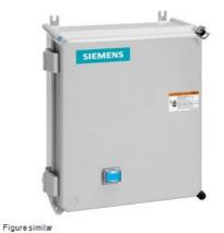
Non-reversing motor starter, Size 1, Three phase full voltage, Solid-state overload relay, OLR amp range 5.5-22A, 110V 50Hz / 120V 60Hz coil, Non-combination type, Enclosure type 4X fiberglass, Water/dust tight noncorrosive, Standard width enclosure
