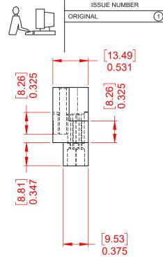
MATERIAL: HOUSING: DIALLYL PTHYHALATE, UL94V-0 CONTACT MATERIAL: COPPER ALLOY CONTACT PLATING: GOLD PLATING OVER NICKEL INSERTION FORCE: 6 TO 16 Oz (0.56 TO 4.45N) PER CONTACT WITHDRAWAL FORCE: 6 TO 16 Oz (0.56 TO 4.45N) PER CONTACT
