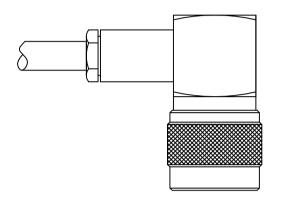
4) Solder the center conductor to the mounting post and screw in the cap.
