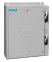
Duplex starter w/o alternator Size 2 Three phase full voltage Solid-state overload relay OLR amp range 13-52A 110VAC 50Hz / 120VAC 60Hz Coil Combination type Two 60A disconnect switches Encl NEMA type 4X 304 S. Steel Water/dust tight non-corrosive
