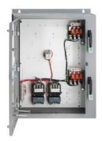
Duplex starter with alternator Size 1.75 Three phase full voltage Solid-state overload relay OLR amp range 10-40A 110VAC 50Hz / 120VAC 60Hz Coil Combination type Two 60A disconnect switches Encl NEMA type 4 painted steel Water/dust tight weather proof
