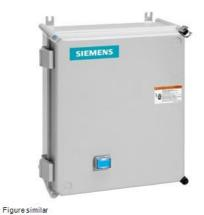
Non-reversing motor starter, Size 1, Single phase full voltage, Solid-state overload relay, OLR amp range 0.75-3.4A, 110V 50Hz / 120V 60Hz coil, Non-combination type, Enclosure type 4X fiberglass, Water/dust tight noncorrosive, Standard width enclosure
