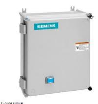
Non-reversing motor starter, Size 0, Three phase full voltage, Solid-state overload relay, OLR amp range 5.5-22A, 208VAC 60Hz coil, Non-combination type, Enclosure type 4X fiberglass, Water/dust tight noncorrosive, Standard width enclosure
