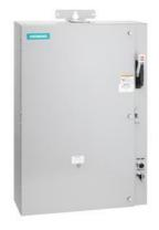
Pump control panel, Size 4, Three phase full voltage, Solid-state overload relay, OLR amp range 50-200A, 24VAC 50-60Hz coil, Standard type contactor, 200A fusible disconnect, 200A/250V fuse clip, HOA Sel Sw. <(>&<)> Start P.B., Enclosure NEMA type 3/3R, Weather proof outdoor use
