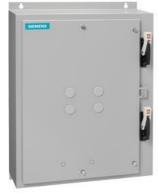
Duplex starter w/o alternator Size 3.5 Three phase full voltage Solid-state overload relay OLR amp range 50-200A Combination type Two 200A disconnect switches Enclosure NEMA type 4/12 Water/dust tight weather proof
