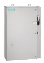
Non-reversing motor starter, Size 3, Three phase full voltage, Solid-state overload relay, OLR amp range 25-100A, Combination type, 125A circuit breaker, Encl NEMA type 4X 316 S-Steel, Water/dust tight noncorrosive, Extra-wide enclosure
