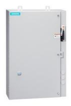
Non-reversing motor starter, Size 1, Three phase full voltage, Solid-state overload relay, OLR amp range 10-40A, Combination type, 30A fusible disconnect, 30A/250V fuse clip, Enclosure NEMA type 4/12, Water/dust tight for outdoors, Extra-wide enclosure
