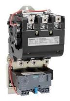
Non-reversing motor starter, Size 3, Single phase full voltage, Solid-state overload relay, OLRelay amp range 25-100A, 110 120/220 240VAC 60HZ coil, Non-combination type, Enclosure type (open), No enclosure
