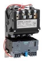
Non-reversing motor starter, Size 2, Single phase full voltage, Solid-state overload relay, OLRelay amp range 25-100A, 24VAC 50-60HZ coil, Non-combination type, Enclosure type (open), No enclosure
