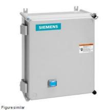
Non-reversing motor starter, Size 1, Three phase full voltage, Solid-state overload relay, OLR amp range 3-12A, 240V 50Hz / 277V 60Hz coil, Noncombination type, Enclosure type 4X fiberglass, Water/dust tight noncorrosive, Standard width enclosure
