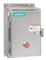
Non-reversing motor starter, Size 0, Single phase full voltage, Solid-state overload relay, OLR amp range 5.5-22A, 24VDC coil, Non-combination type, Encl. type 4X 304 S. Steel, Water/dust tight noncorrosive, Standard width enclosure
