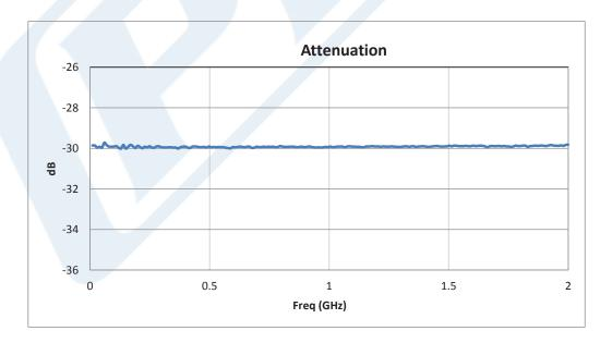
Click the following link (or enter part number in "SEARCH" on website) to obtain additional part information including price, inventory and certifications: 30 dB Fixed Attenuator, BNC Male to BNC Female Brass Nickel Body Rated to 1 Watt Up to 2 GHz PE7000-30
