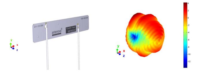
**3D pattern at 1575 MHz**Drag to rotate pattern and PCB by using Adobe Reader
