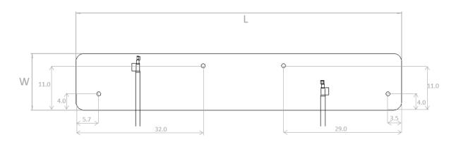
$4 \text{ Holes} = 1 \text{mm } \emptyset \text{ (diameter)}$
