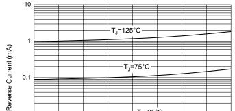
Fig. 6 - Typical Reverse Leakage Characteristics
