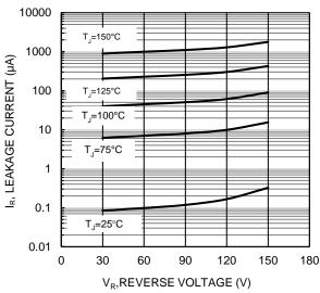
Figure 3. Typical Reverse Characteristics
