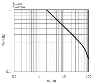
Figure 6. Normalized Avalanche Power Derating Versus
