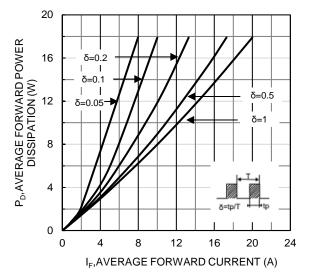
Figure 1. Forward Power Dissipation
