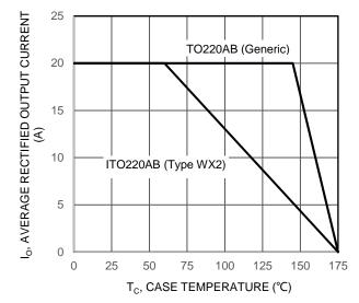
Figure 4. DC Forward Current Derating
