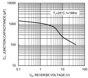
Figure 5. Typical Reverse Characteristice
