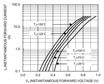
Figure 2. Typical Forward Characteristics
