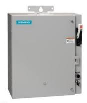
Pump control panel, Size 2, Three phase full voltage, Solid-state overload relay, OLR amp range 13-52A, 220-240/440-480VAC 60Hz coil, Standard type contactor, 50A circuit breaker, HOA Sel Sw. <(>&<)> Start P.B., Enclosure NEMA type 3/3R, Weather proof outdoor use
