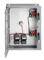
Duplex starter with alternator Size 2 Three phase full voltage Solid-state overload relay OLR amp range 13-52A 110VAC 50Hz / 120VAC 60Hz Coil Combination type Two 60A disconnect switches Enclosure NEMA type 1 Indoor general purpose use
