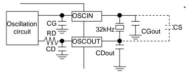
\*1) The CGOUT or/and CDOUT should have a capacitance ranging from 0 to 6 pF. (Including parasitic capacitance of the printed circuit board)
