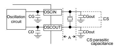
Typical externally-equipped element X'tal : 32.768kHz ECO mode OFF: Max. R1 up to  $80k\Omega$ ECO mode ON : Max. R1 up to  $65k\Omega$ CL=6 to 12.5pF CGOUT=CDOUT=0pF Standard values of internal elements CG, CD 10pF typ.
