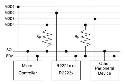
\* For data interface, the following conditions must be met: VCC4≥VCC1 VCC4≥VCC2 VCC4≥VCC3
