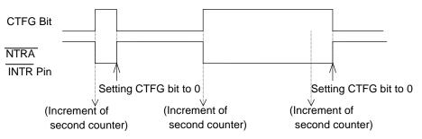
\*1), \*2) When the oscillation adjustment circuit is used, the interrupt cycle will fluctuate once per 20sec. as follows:
