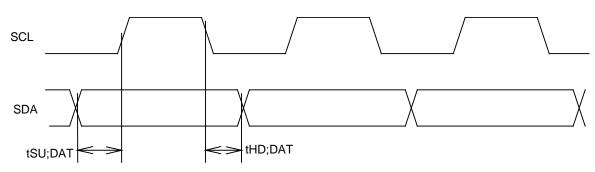
The SCL and SDA pins are at the "H" level when no data transmission is made. Changing the SDA from "H" to "L" when the SCL and the SDA are "H" activates the Start Condition and access is started. Changing the SDA from "L" to "H" when the SCL is "H" activates Stop Condition and accessing stopped. Generation of Start and Stop Conditions is always made by the master (see the figure below).
