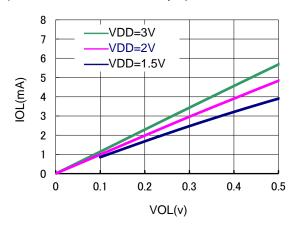
Vol vs lol (SDA pin) 8 6 VDD=3V 6 VDD=2V 6 VDD=1.5V 2
