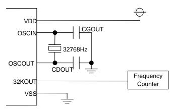
X'tal: 32.768kHz  $(R1=30k\Omega typ)$ (CL=7pF) Topt : 25°C Output pins : Open
