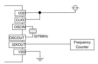
\* 1) The R2221x, R2223x is configured to generate 32.768-kHz clock pulses for output from the 32KOUT pin.
