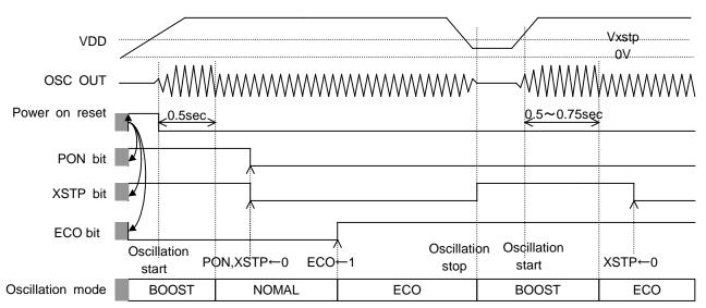
\*) The power on reset shown above is an internal signal and the signal is generated from right after the VDD turns on until the oscillation of quartz crystal unit starts. While the term of the power-on reset signal is out, or the time until the oscillation of quarts crystal unit starts, approximately 0.1s to 1.0s, access of I2C bus is impossible.
