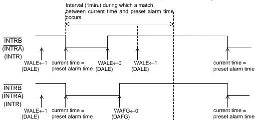
After setting WALE(DALW) to 0, Alarm registers is set to current time, and WALE(DALE) is set to 1, INTRB (INTRA) will be not driven to "L" immediately, INTRB (INTRA, INTR) will be driven to "L" at next alarm setting time.
