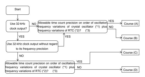
\* 1) Generally, quartz crystal units for commercial use are classified in terms of their center frequency depending on their load capacitance (CL) and further divided into ranks on the order of  $\pm 10$ ,  $\pm 20$ , and  $\pm 50$  ppm depending on the degree of their oscillation frequency variations.
