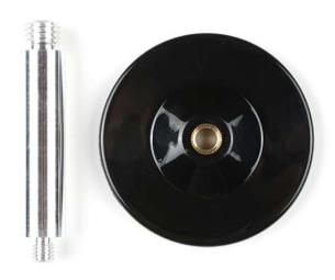
This is a very handy magnetic mount for survey grade GNSS/GPS antennas. Sturdy, compact, and surprisingly strong, this is a quick way of mounting your antenna to metal roofs, parapets, and other ferrous materials. The rod is threaded 5/8" 11-TPI (threads per inch) found on high-end surveying antennas and equipment. Additionally, the mount is tall enough to prevent kinking or collision between the TNC connector, cable, and the roof surface.
